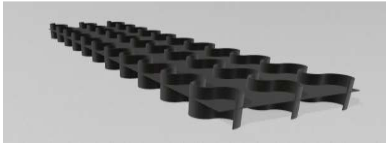
Figure 3: The general geometry for wave fins attached to both side of absorber (upper and lower)
